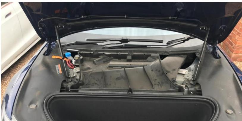
The lower cover has two breather pipes that also need to be removed. They simply pull off.
