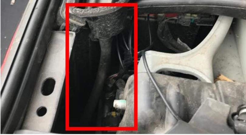
Remove the air scoop. The mountings are located at either end.
