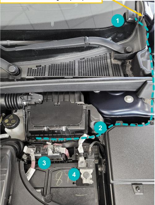
Remarks: To access the +12V connection, remove the black and red plastic cover. Make sure that the plastic cover is put back correctly.
