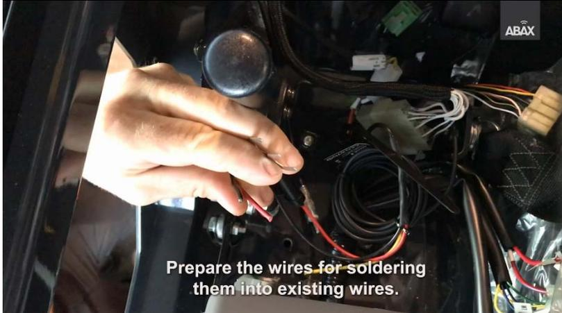
Use a solder iron or an appropriate connecting tool to connect the red wire to a permanent feed, black to ground and yellow to an ignition source. Where appropriate, cover with heat shrink tubing to prevent short-circuiting.
